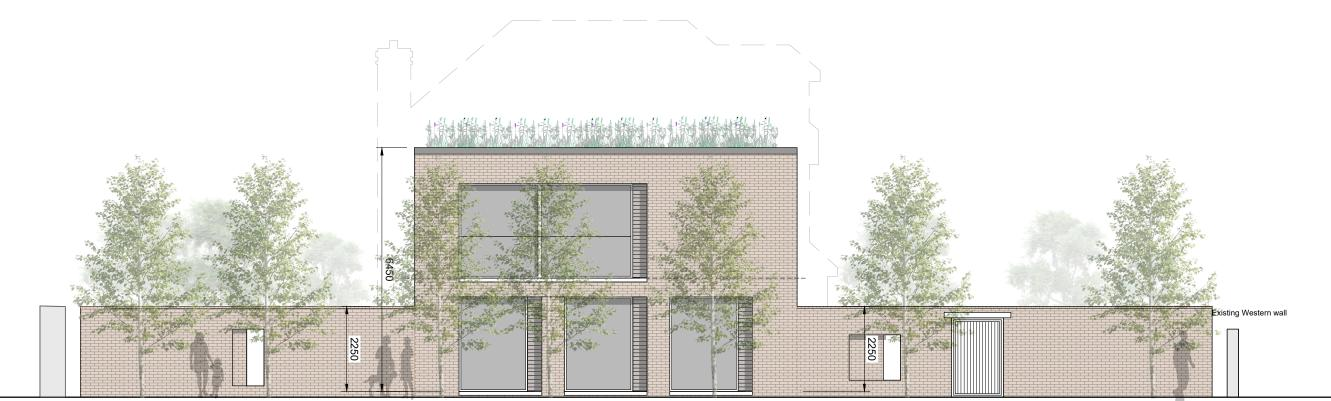
Gap of aprox 400mm between proposed wall and Existing Eastern wall to allow for glimpse through to courtyard.
